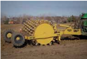
ROLLING PACKER PULL-TYPE WITH HYDRAULIC LIFT SYSTEM
