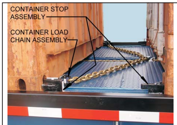
Figure 3-7 Loading Two Containers
